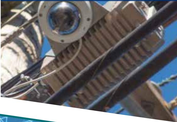
An Alpha XM gateway enables Wi-Fi, small cell or IP camera backhaul at the power supply.
