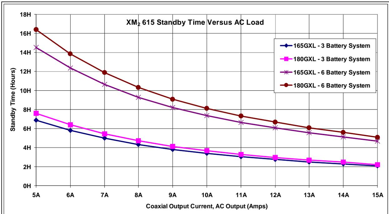
Figure 5. AlphaCell 180GXL and 165GXL battery run times for different XM<sub>2</sub> output currents loads into the CATV plant.
