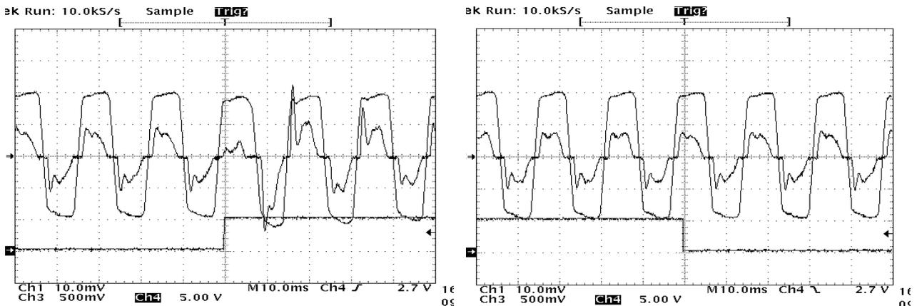
Figure 1. Examples of XM<sub>2</sub> transitions between utility powering and standby powering using CATV load.
