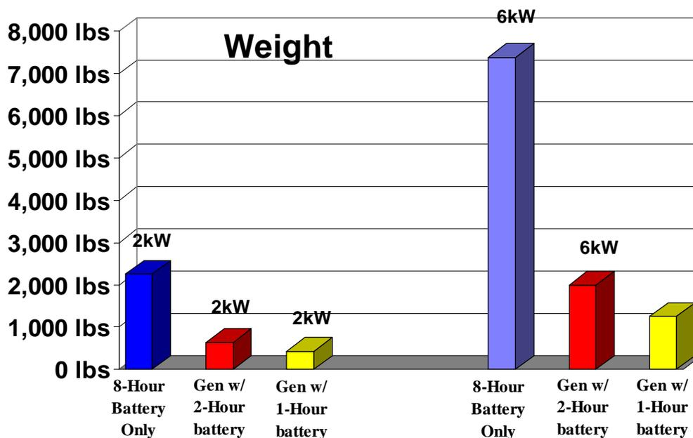
Figure 4. Comparison of weight by different energy-storage systems.
