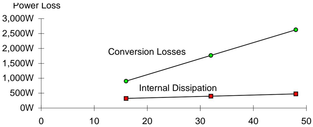
**Figure 5.** Power losses in an RT versus quantity of ONU-48s hosted.
