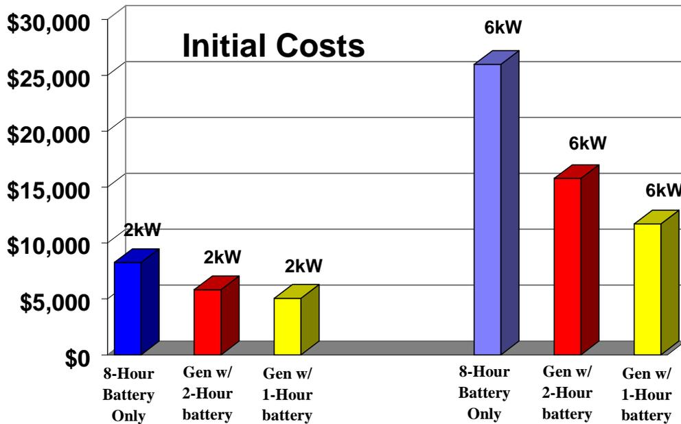
**Figure 1.** Comparisons of initial cost for two power levels, 2kW and 6kW. Comparisons are made among an eight-hour, battery only solution, and combination of generator and a one-hour and two-hour battery backups.
