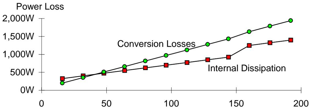
**Figure 6.** Power losses in an RT versus quantity of ONU-24s hosted.
