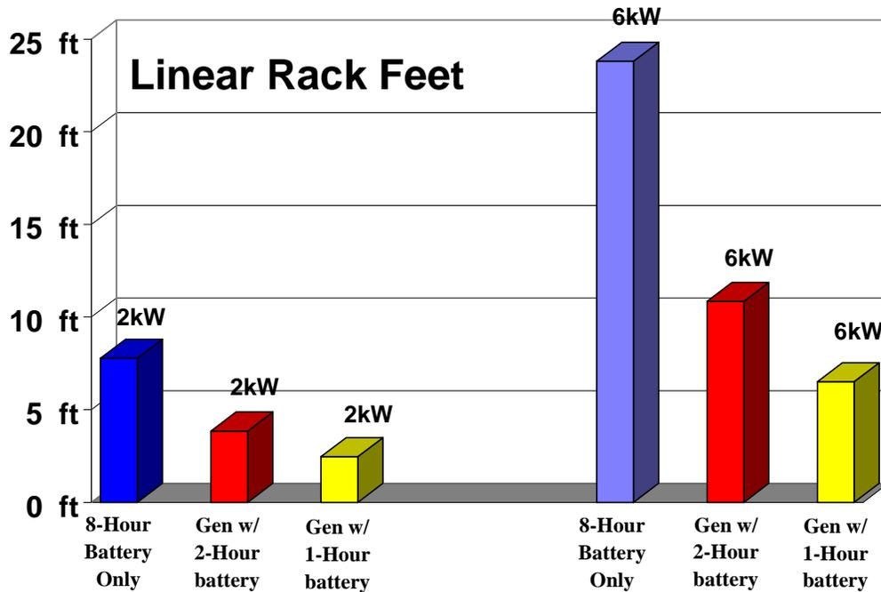
**Figure 3.** Comparison of physical size occupied by different dc energy-storage systems: eight-hour of battery only, a two-hour battery plant with an engine generator, and a one-hour battery plant with an engine generator.
